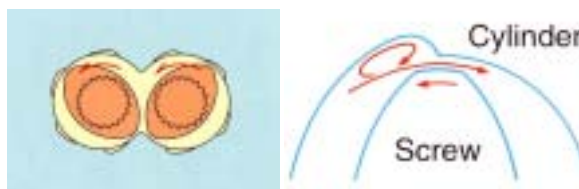
Fig. 5 Special kneading cylinder "NIC"
