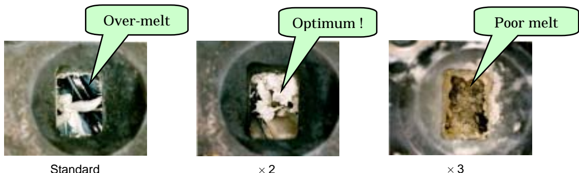
Photo 1 Observation of material condition through the vent opening (PP+60%TiO 2 )
